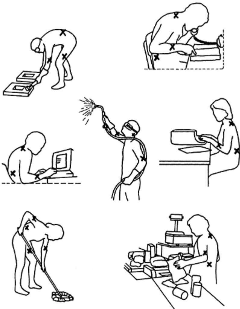
FIGURE 9.3 Examples of work postures where there are problems with extreme joint angle, large muscular force, high degree of repetition, or high contact pressure (from Webb, 1982).
