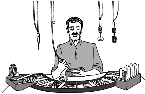
FIGURE 20.14 Workplace arrangement of tools and bins. (Adapted from International Labour Office, Introduction to Work Study , third ed., International Labour Office, Geneva, Switzerland, 1986.)
