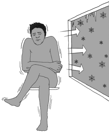
FIGURE 8.2 Heat radiated from the body to a cold window-pane. (Adapted from Kroemer, K. H. E., and Kroemer, A. D., Office Ergonomics , Korean edition, Kukje Publishing, Seoul, South Korea, 2006.)
