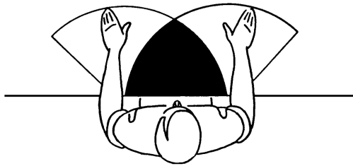
FIGURE 20.12 Work area suitable for finely controlled manipulation. (Adapted from International Labour Office, Introduction to Work Study , third ed., International Labour Office, Geneva, Switzerland, 1986.)
