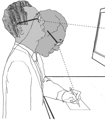
FIGURE 5.3 Excessive eye/head/neck movements can be avoided by placing visual targets close to each other. (Adapted from Kroemer, K. H. E., and Kroemer, A. D., Office Ergonomics , Korean edition, Kukje Publishing, Seoul, South Korea, 2006.)
