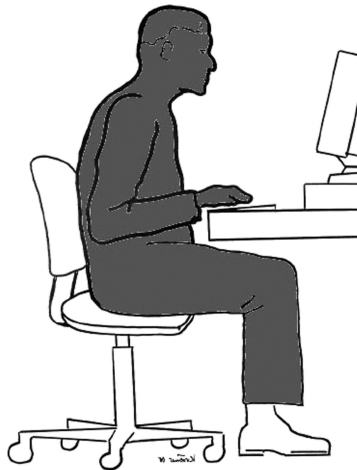
FIGURE 18.11 The monitor is set up too far from the eyes and too high, so the operator arches his back and neck in trying to get the image into focus. (Adapted from Kroemer, K. H. E., and Kroemer, A. D., Office Ergonomics , Taylor & Francis, London, 2001.)
