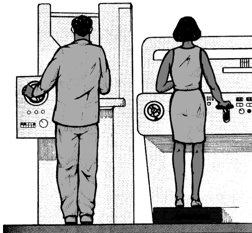
FIGURE 20.3 Use of a platform to stand on can be of help to a shorter person to operate a machine designed for a taller operator. (Adapted from International Labour Office, Introduction to Work Study , third ed., International Labour Office, Geneva, Switzerland, 1986.)
