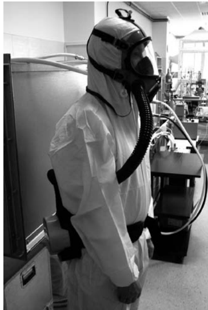
FIGURE 26.18 Powered filtering device incorporating a helmet or a hood and power-assisted filtering device incorporating full face mask, half mask, or quarter mask.
