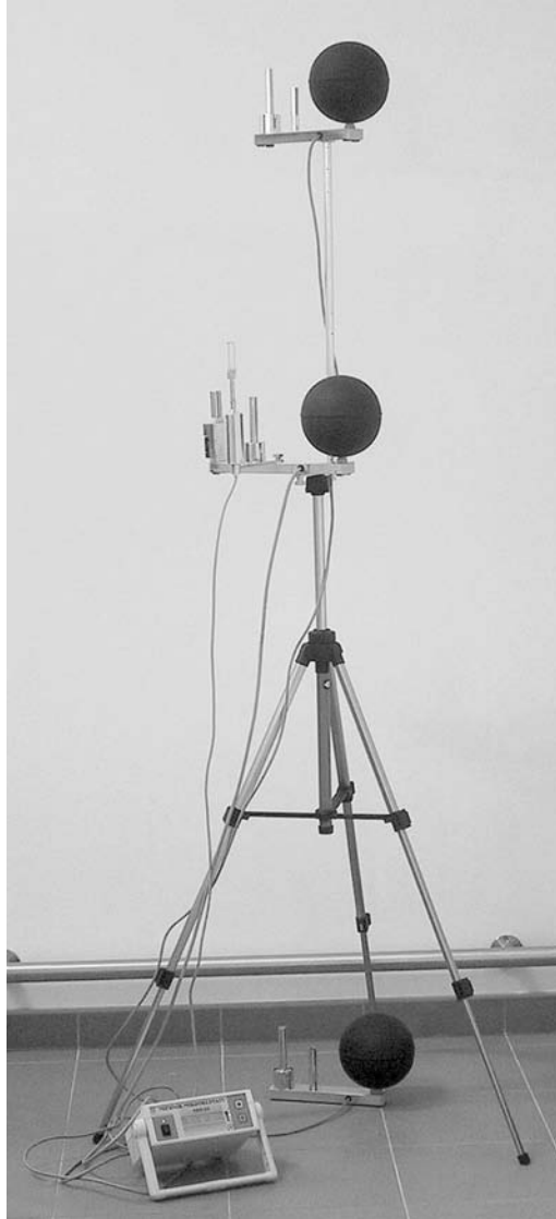
FIGURE 16.4 Set of three sensors for measuring air values in heterogeneous thermal conditions.
