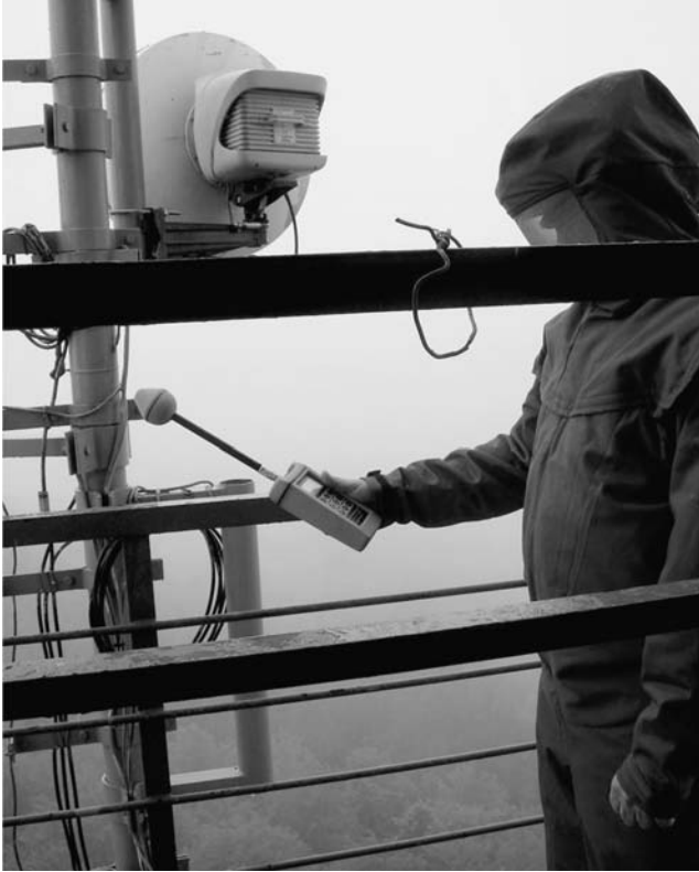
FIGURE 9.12 Suits protecting workers against electromagnetic field exposure, designed by CIOP-PIB researchers.
