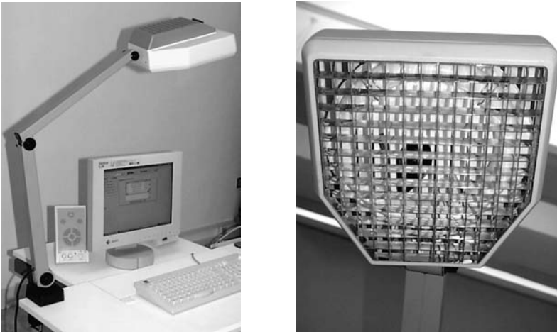
FIGURE 12.8 An example of a task lighting luminaire suitable for illuminating a computer workstation and a view of a parabolic mirror louver that provides antiglare shielding.
