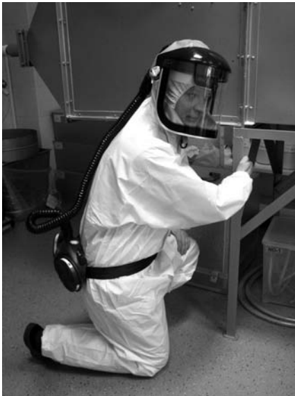
FIGURE 26.18 Powered filtering device incorporating a helmet or a hood and power-assisted filtering device incorporating full face mask, half mask, or quarter mask.
