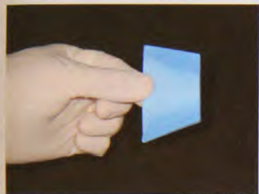
FIGURE II-3 Shine produced by even heating on the edges.
