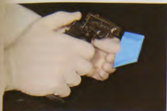
FIGURE II-2 Using a torch to soften the wax.
