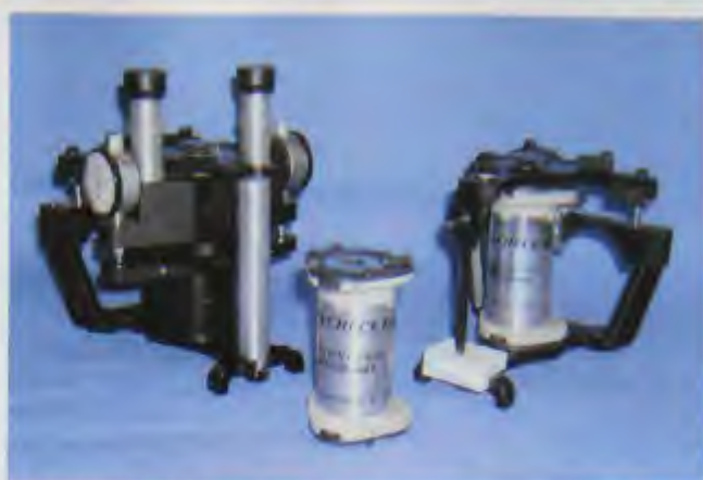
FIGURE 22-28 Dénar ® (Water Pik, Inc.) field gauge (left), and the Check Key (right). Such devices ensure interchangeability of articulators without loss of accuracy.
