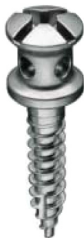
Fig. 7. The screw used in the proposed case has the following features: 2.0mm screws, 8-12mm thread lengths, made of 316L extra-hard stainless steel for maximum strength; self-drilling, self-tapping for one-step insertion; groove under screw-head secures wires or elastics; cruciform head design; two cross-holes with align cruciform head slots; a 4-mm capstan-style head to hold the wire away from the mucosa (Synthes, West Chester, Pennsylvania).
