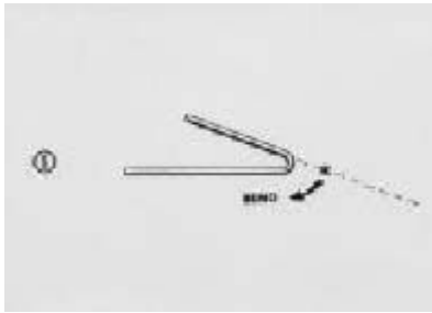
Figure 37. The helical loop spring construction is begun by bending the 0.022" wire with the conical beak of a #139 pliers.
