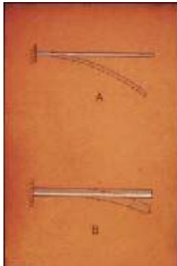
Figure 45. The thin wire A) must be deflected more than the thick wire B) to produce the same amount of force.
