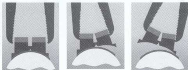
Figure 14-8 A ceramic bracket design showing a vertical scribe line placed in the base of the appliance for ease of removal or debonding. (Courtesy Unitek Corporation/3M, Monrovia, Calif.)
