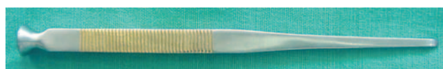
Fig. 7.11: Chisel for bone removal. The width of tip varies from 3 to 6 mm. Stainless steel chisels require frequent sharpening while those with tungsten carbide tips retain their sharpness for a longer time
