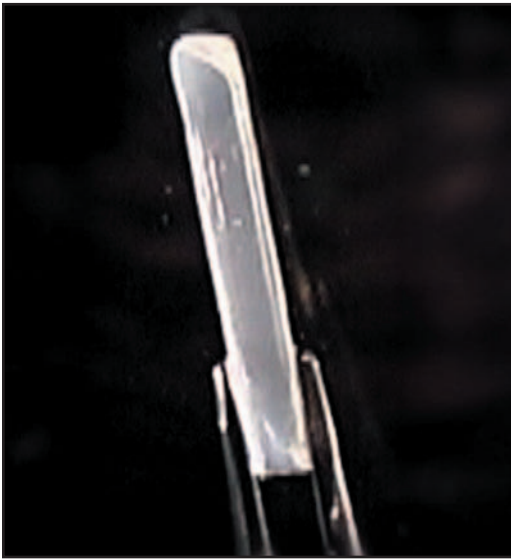
Figure 26-2. Photograph illustrating design characteristics and experimental performance of the one-piece SmartIOL. At room temperature, the SmartIOL biomaterial is formed into a solid rod of approximately 30.0 mm length and 2.0 mm width. There is a transformation of the rod into a biconvex lens, after immersion in BSS at body temperature.
