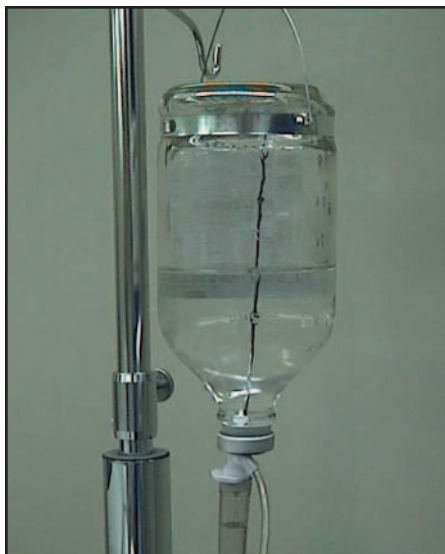
Figure 8-1. Air tubing connected from the air pump of a fish tank into the drip chamber of the irrigation administration set.
