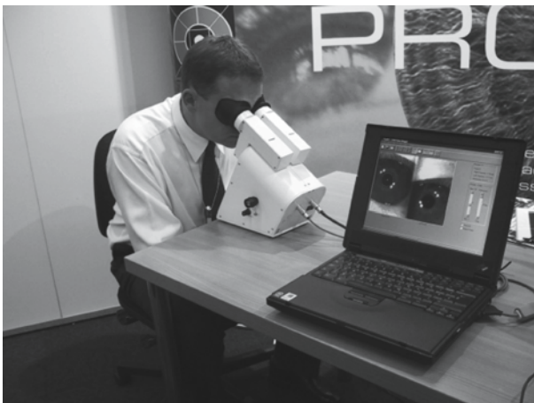
Fig. 18.5. Bilateral pupillometry utilising the Procyon bilateral simultaneous infra-red digital pupillometer. Patient's eyes fixed onto rubber cups to exclude external light
