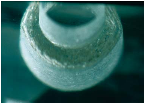
Fig. 10.19. Macrophotograph of inverse mushroom shaped trephination using a femtosecond laser [67]
