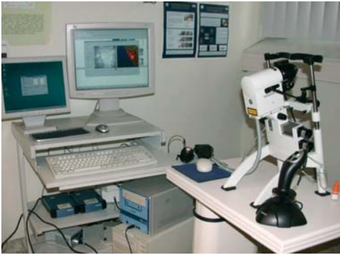
Fig. 13.5. Rostock Cornea Module (RCM) (confocal laser-scanning microscope)
