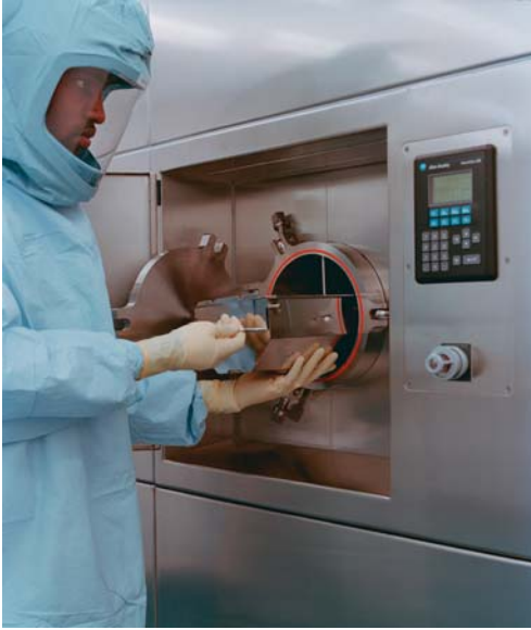
Fig. 1.3. The BioCleanse sterilization process involves use of various chemical solutions, cycles of pressure and vacuum, and serial dilution to inactivate and remove pathogens including bacteria, viruses, spores, and fungi. (Photograph courtesy of Regeneration Technologies, Inc.)
