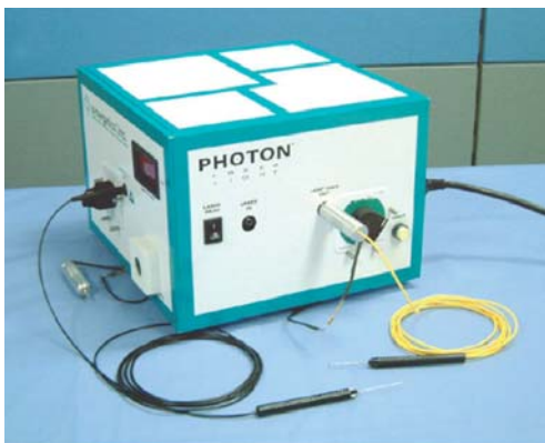
Fig. 7.3 Xenon light source. Both can provide enough illumination for detailed observation in the 25-gauge system
