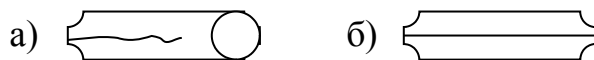
Fig. 1.3. Discharge meters: a) end; b) cylindrical Semiconductor (crystal) meters are also ionization meters in which a flying particle generates conduction electrons and "holes" in the semiconductor.
