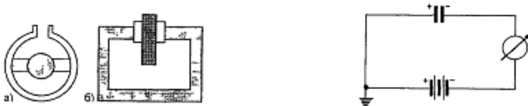
Fig. 1.6. Ionization chamber Fig. 1.7. Electrical diagram of the ionization chamber Radioluminescent (photoluminescent and thermoluminescent) method
