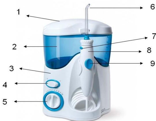
Fig. 1. The general structure of a stationary irrigator: 1- cover of the water tank with a compartment for storing nozzles; 2 - water tank; 3 - base; 4- on/off button; 5 - pressure regulator; 6 – nozzle; 7- nozzle release button; 8 – handle; 9 – pause button.
