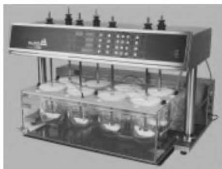
Fig. 3 Installation for testing for dissolution of tablets and capsules manufactured by Pharmatest (Germany) model PTWS 3CE
