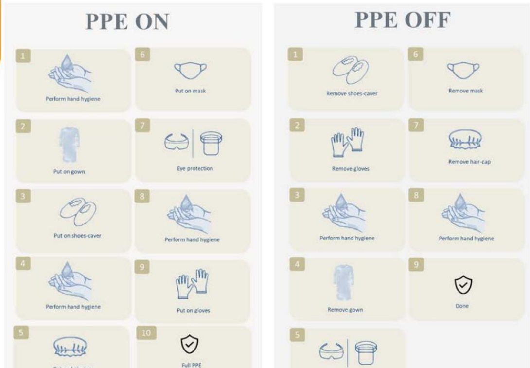
Figure 7. Principle of Personal Protective Equipment on and off techniques
