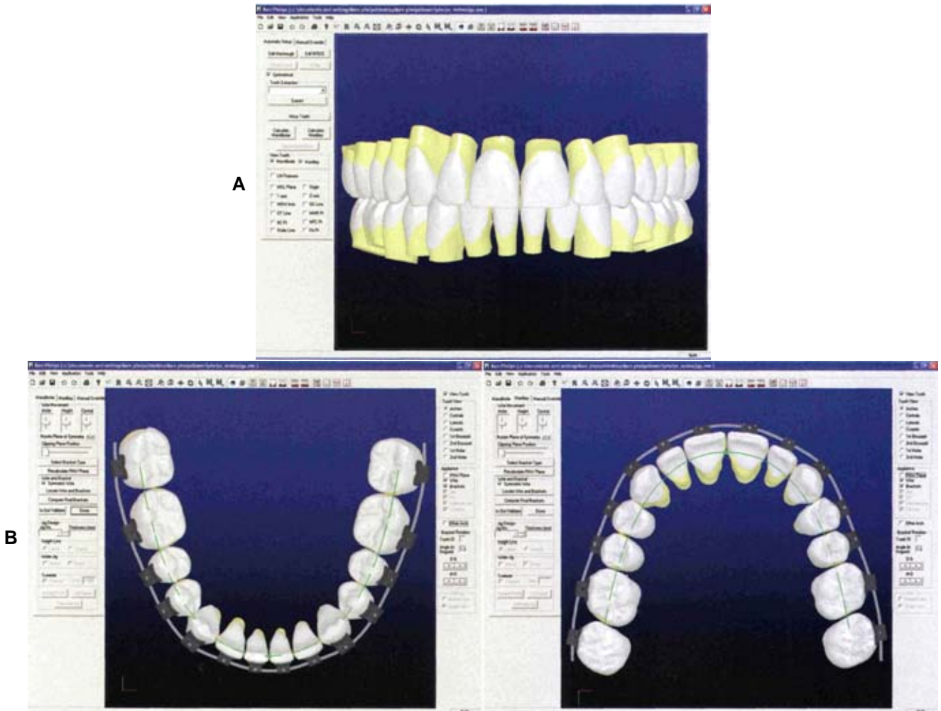
FIGURE 11-37 A, The preparation of Insignia custom facial brackets (Ormco) begins with a laser scan of the patient's dental casts, so that the contours of the individual teeth are captured in computer memory and the teeth are reset to ideal position. B, C, The base for each individual bracket is milled to fit a specific tooth, and the bracket slot is cut to match the ideal position of that tooth with a rectangular archwire in place. The goal is to have a final rectangular archwire that requires no chairside fabrication to produce ideal tooth positions. (Courtesy Ormco/Sybron.)
