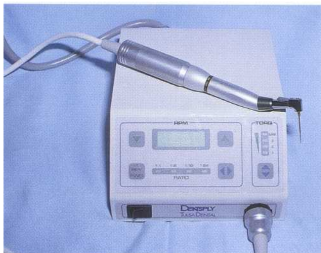
FIGURE 5-1 A high-torque, low-rpm electric handpiece designed for nickel-titanium rotary instrumentation.
