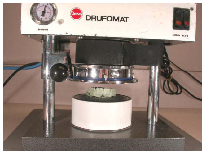
Figure 11-29 Heating element in position over the model allowing the EVA material to heat up.
