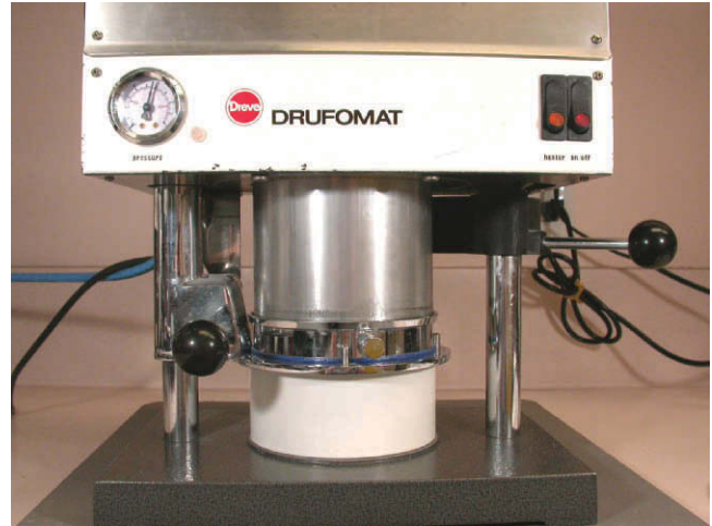
Figure 11-33 A proper cool down period of 10 minutes prevents distortion.
