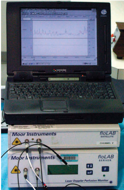
Figure 6-20 When properly used, laser Doppler flowmetry will indicate as early as 2 to 3 weeks posttrauma if revascularization is occurring.
