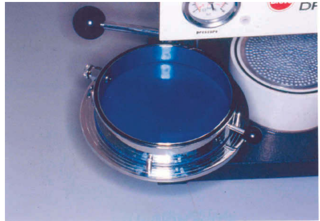
Figure 11-28 A clamping ring locks the EVA sheet into place.
