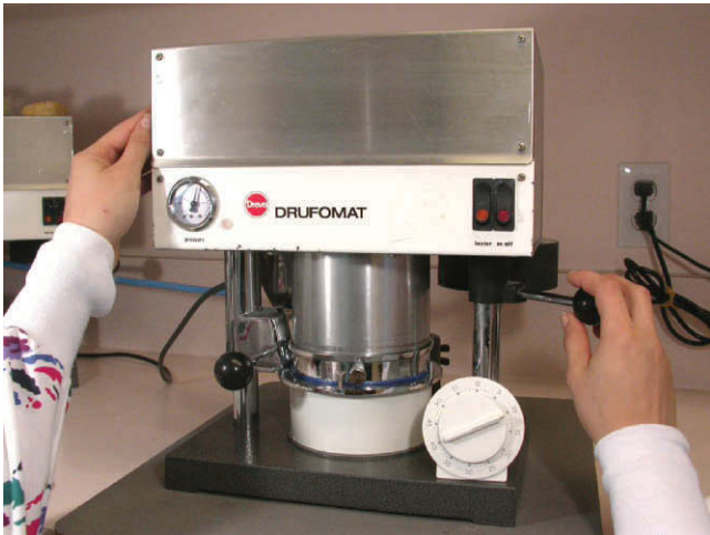
Figure 11-32 Pressure is used on the first layer and timing is critical to maintain pressure while cooling.
