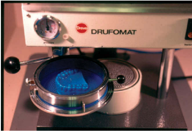
Figure 11-36 Completed pressurized and cooled first layer.
