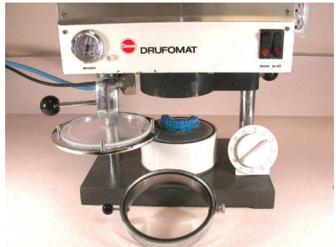
Figure 11-44 Preparation for second layer placement of EVA material. Note the second layer is clear.
