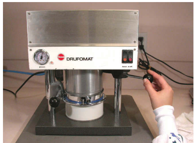
Figure 11-35 The heater lever is slowly pushed toward the cylinder until the cylinder rises.
