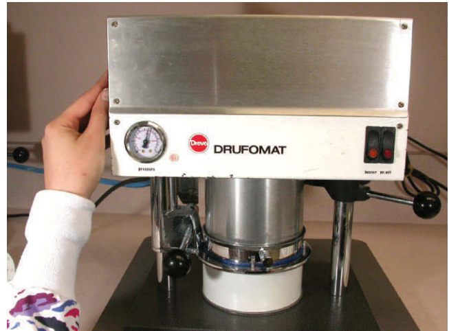
Figure 11-34 White button on side panel is pressed until pressure indicator light is turned off.
