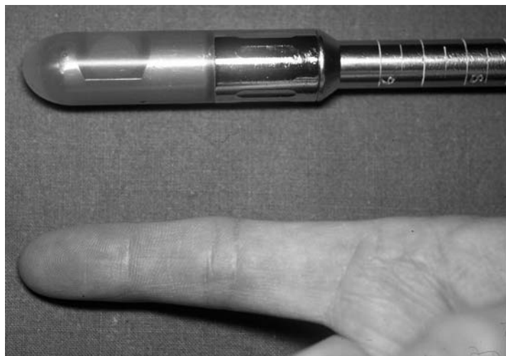
FIGURE 11.14. The transducer protected by a plastic cone.
