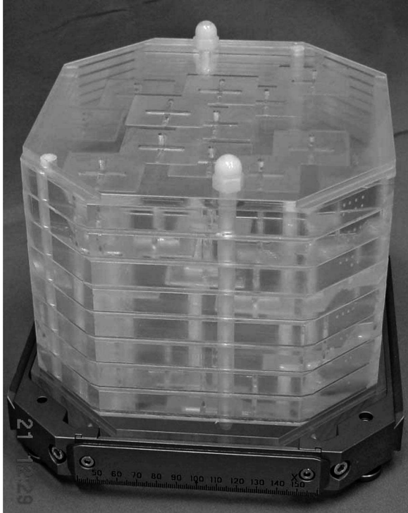
Fig. 1. Known target point phantom used in MR imaging, consisting of 8 lucite plates with 21 imbedded 3D cross hairs, mounted in the stereotactic Leksell frame.
