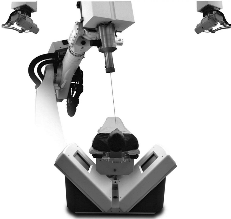
Fig. 1. The CyberKnife radiosurgical system. Note the two amorphous silicon X-ray screens positioned orthogonally to the treatment couch. The couch can move to position the fiducials in front of the cameras. The CyberKnife consists of a linear accelerator mounted on a 6-axis robotic manipulator that permits a wide range of beam orientations.
