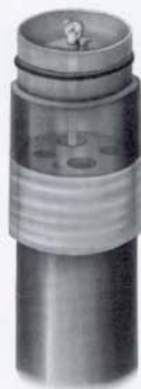
Fig. 95 Cylinder assembly. The outer cylinder is attached to the tip of the endoscope. The trip wire is connected to the inner cylinder, which is loaded with the rubber band. The trip wire runs throughout the length of the endoscope working channel.
